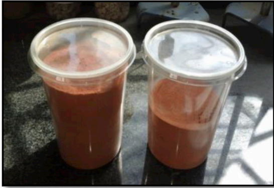
Fig. 1. Pottery Powder passed through a No. 200 sieve (75 \mu\text{m} ).
