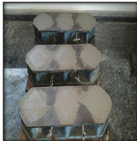
Fig. 5. Moulds used to preparation mortar specimens.
