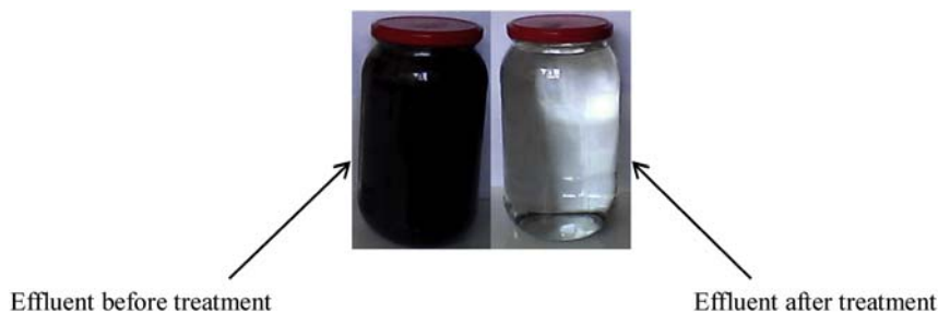
Fig. 6. Mineral oil effluent before and after electrocoagulation treatment.
