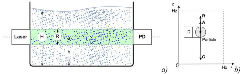
Fig. 1. The measurement system scheme (a); the forces acting on the particle in a liquid (b);  $\mathbf{G}$  is the gravity force,  $\mathbf{A}$  is the Archimedes force,  $\mathbf{R}$  is liquid resistance force,  $D$  is the diameter of the particle.
