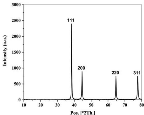
Fig. 4. X-ray diffraction (XRD) profile of crystalline LA-AuNPs.
