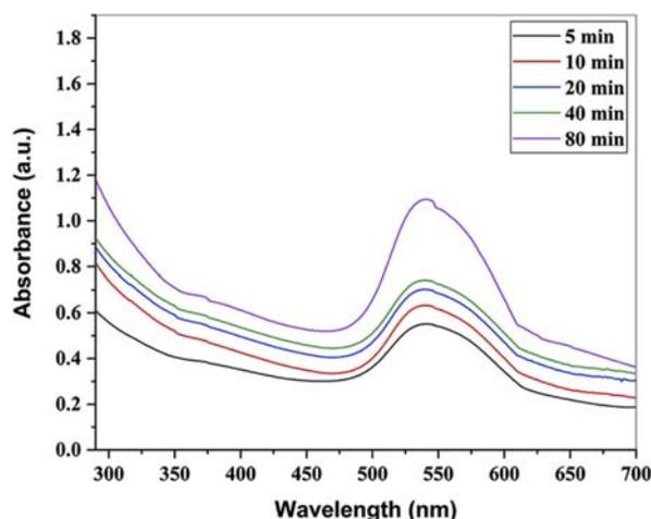
Fig. 1. UV–vis absorption spectra of the formed LA-AuNPs.
