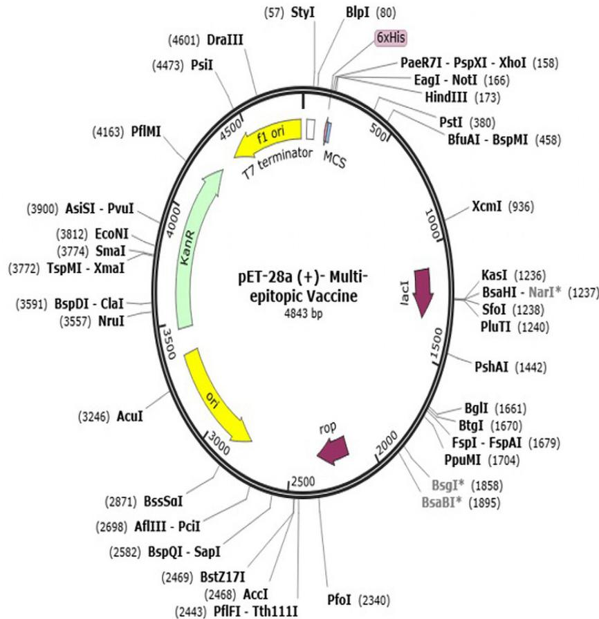
Fig. 7. Showing the insertion of multiepitope vaccine in pET-28-a(+) expression vector between HindIII and NaeI and found in results a colon of 4843bp.
