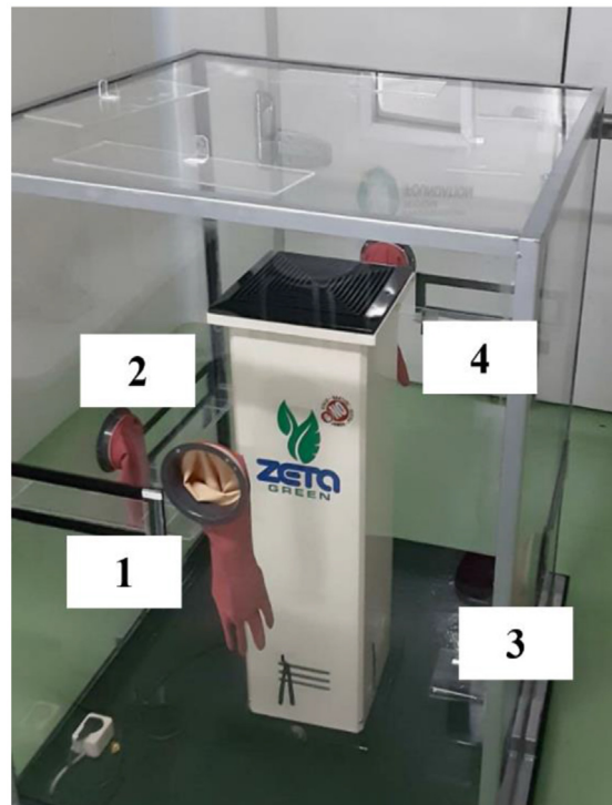
Fig. 1. A CPE is put in a test chamber for experimental transmission of SARS-CoV-2 through airborne in the chamber. This test chamber was built as a BSL3 facility. The test chamber is free from contamination when the stained plates are inserted into the test chamber. Indications with numbers 1, 2, 3, and 4 show the shelves on which to place Petri dishes containing serum with SARS-CoV-2 contamination in the chamber test.
