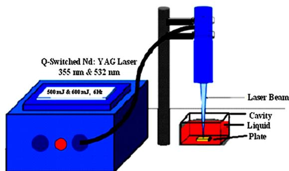
Fig. 2. Schematic diagram of PLAL for NPs synthesized.
