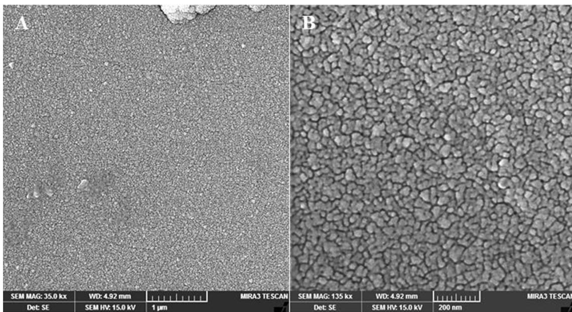
Fig. 8. SEM images of ZnNPs at 532 nm-600 mJ-900 P zoom (A) 1 μm (B) 200nm.
