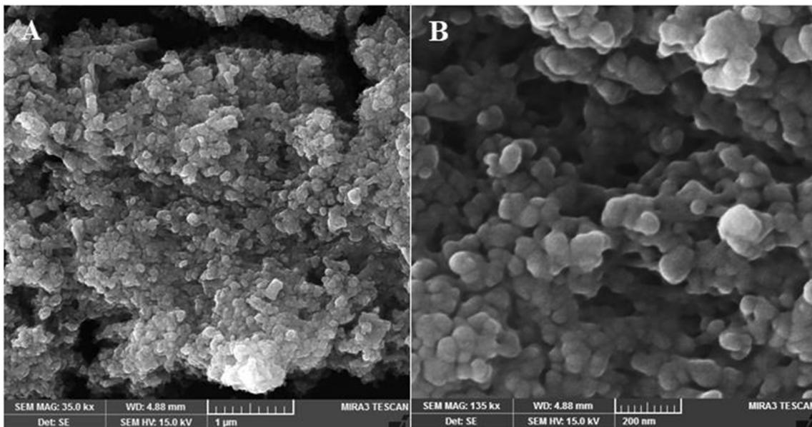
Fig. 6. SEM images of ZnNPs at 355 nm-500 mJ-900 P zoom (A) 1 μm (B) 200nm.
