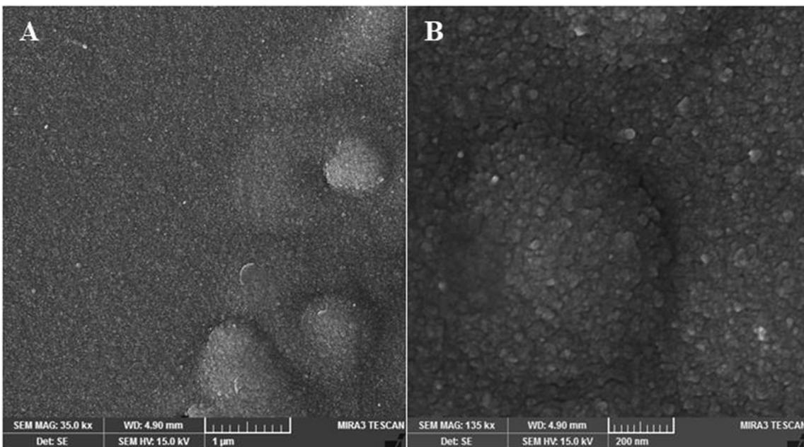
Fig. 7. SEM images of ZnNPs at 532 nm-600 mJ-800 P zoom (A) 1 μm (B) 200nm.
