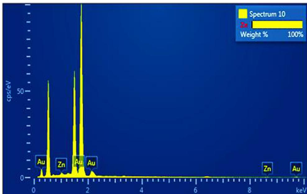
Fig. 11. EDX analysis at 532nm-900P.
